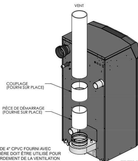
LE TUYAU DE 4" CPVC FOURNI AVEC LE CHAUDIÈRE DOIT ÊTRE UTILISÉ POUR LE RACCORDEMENT DE LA VENTILATION
